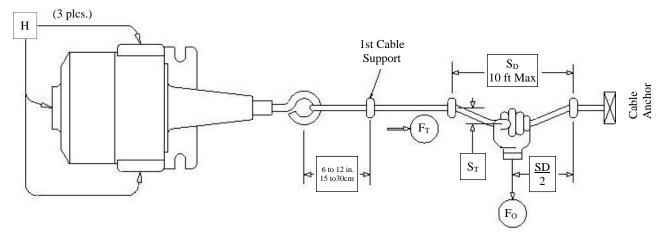
$F_T$  = The value of force, along the cable, which trips the switch.
