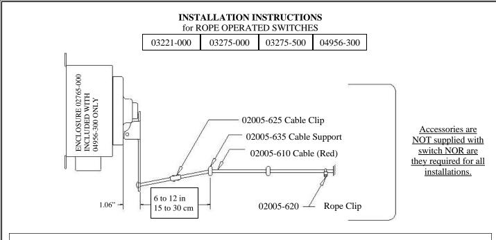
Since every installation is unique and separate, the following instructions can be considered flexible. There are some basic switch setup procedures that must be observed and they are indicated by the symbol (≻). The balance of the suggestions and information is subject to change to accommodate those most familiar and responsible for the installation.
