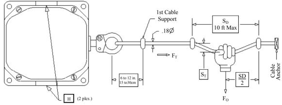
$F_T$ = The value of force, along the cable, which trips the switch.
